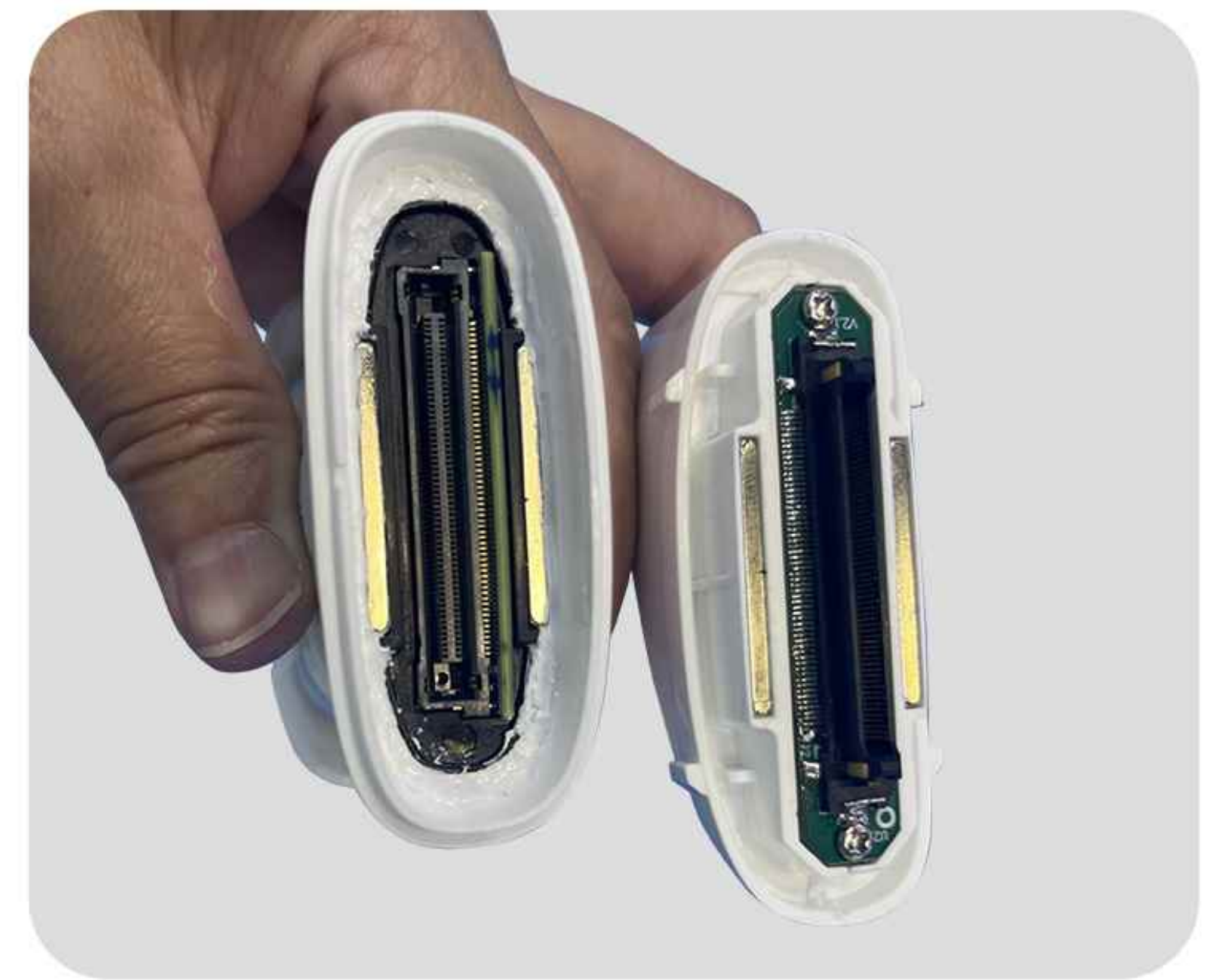
The transducer and the handle are precisely and magnetically connected
